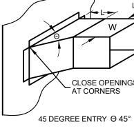
EXPANSION CLEARANCE SHALL BE A MINIMUM OF 3mm (1/8") PER FOOT OF WIDTH OR HEIGHT OF THE SLEEVE TO A MAXIMUM OF 38mm (1 1/2") AND A MINIMUM OF 6.25mm (1/4")
